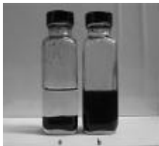
CNT nanofluids with and without dispersant: (a) NTs quickly settle without use of a proper dispersant, and (b) NTs are well dispersed and suspended in the oil with succinimide dispersant (5 wt.%).
