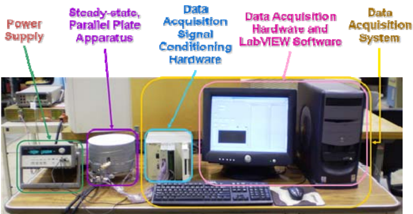
Steady-state, Parallel-Plate Thermal-Conductivity (PPTC) apparatus [4]
