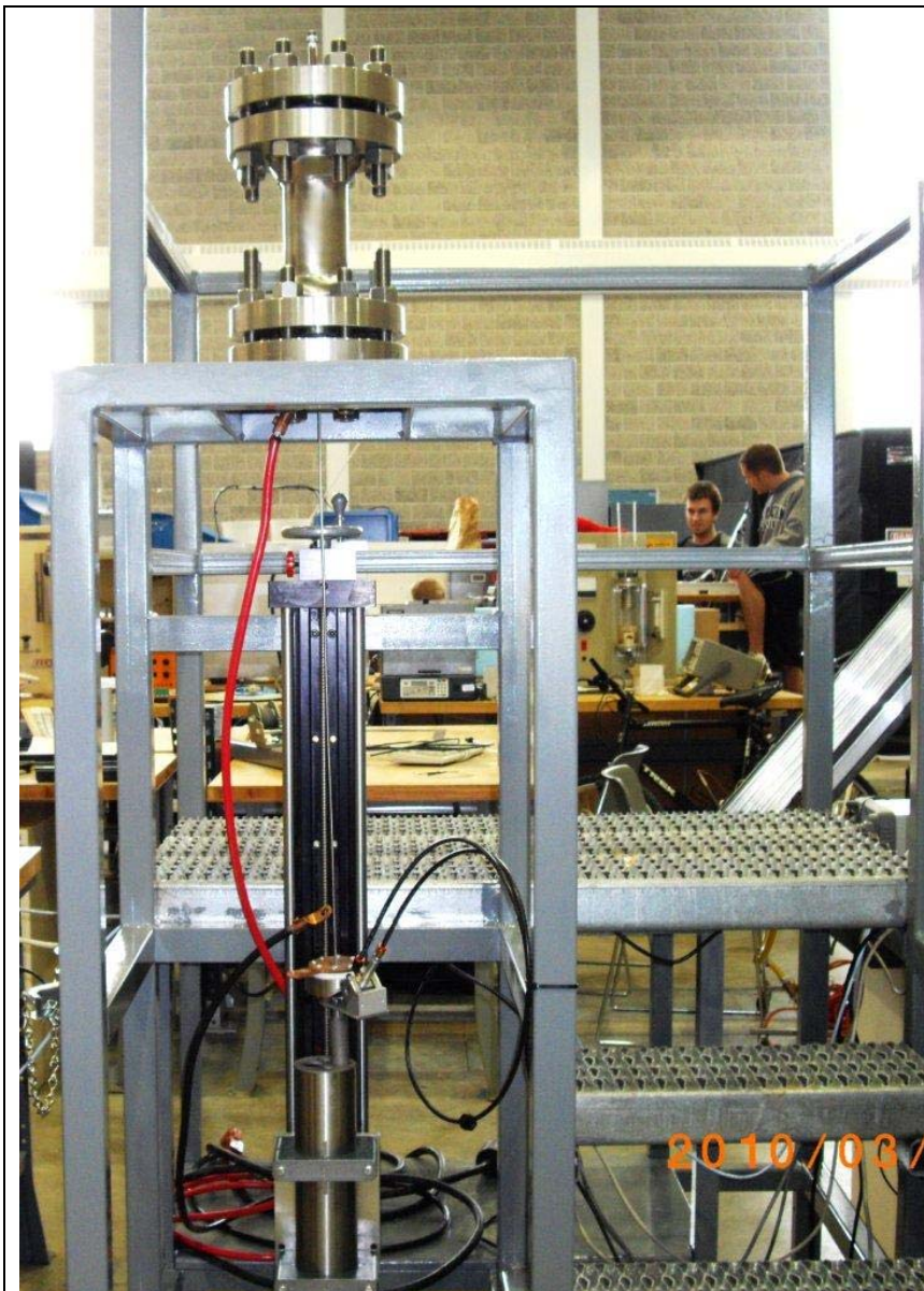
Flow and heat Transfer apparatus for nanofluids (n-FHT Apparatus)
