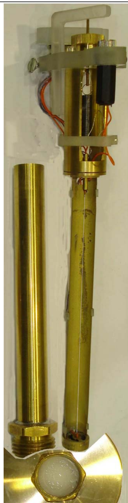
Transient Hot-Wire Thermal Conductivity (HWTC) apparatus [3]
